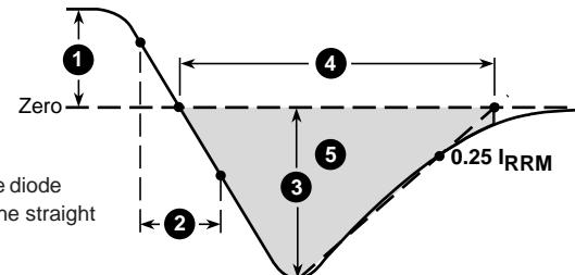
Figure 10. Diode Reverse Recovery Waveform and Definitions
