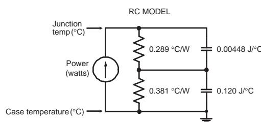
FIGURE 1b, TRANSIENT THERMAL IMPEDANCE MODEL
