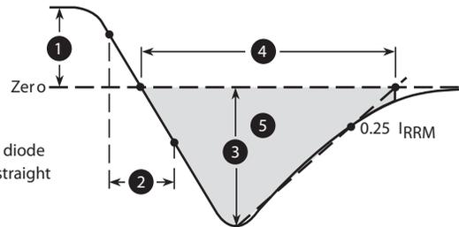
Figure 10. Diode Reverse Recovery and Definitions
