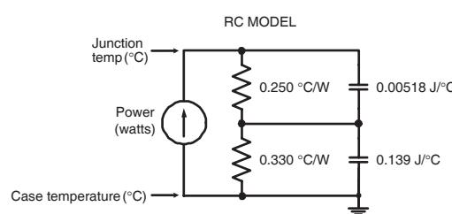
FIGURE 1b, TRANSIENT THERMAL IMPEDANCE MODEL
