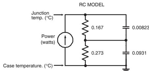
FIGURE 1b, TRANSIENT THERMAL IMPEDANCE MODEL
